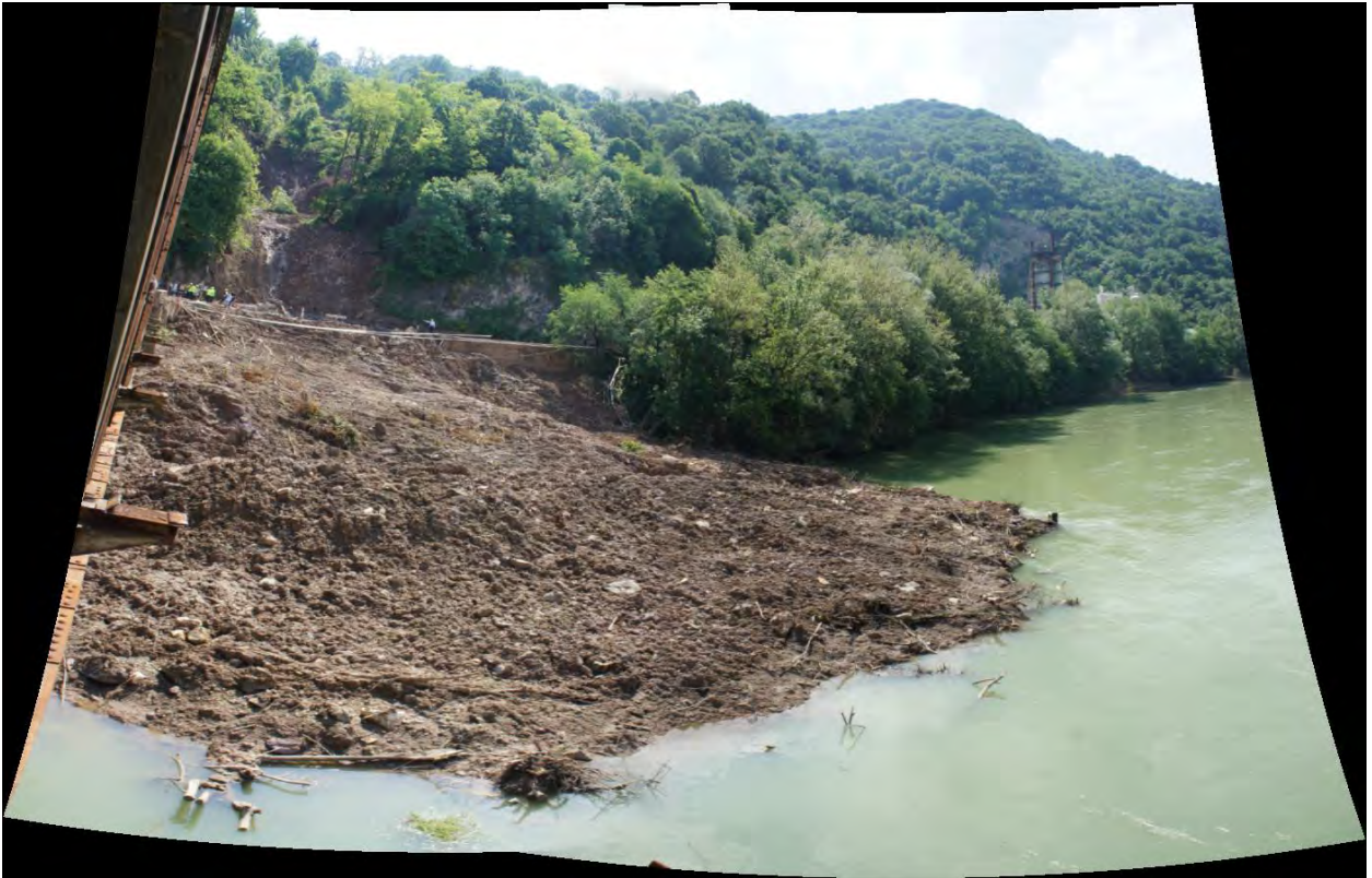
Figure 4.4 - View from pedestrian bridge looking west to the debris flow at the toe of the Mali Zvornik landslide.
