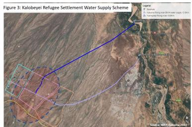
shallow boreholes with an average depth of 30 meters in Kamnyaep area along the Tarach river basin. The source of water is 10.8 km away from the Kalobeyei Refugee Settlement, and It is characterised as high yielding, shallow
